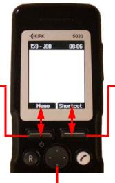
Right Softkey Pressing right softkey activates right softkey text.
